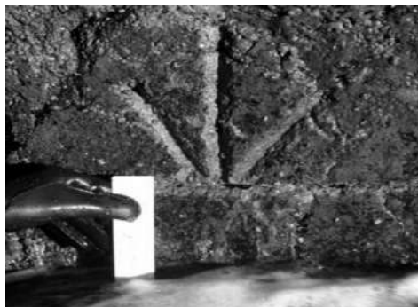
Figure 102. Zoom on the etched benchmark displayed in the ellipse (near center-left) of Figure 101, that was engraved under the order of Capt. Sir James Clark Ross in 1841 to indicate the mean sea level at the Isle of the Dead (Tasmania). After Hunter et al. (2003).
